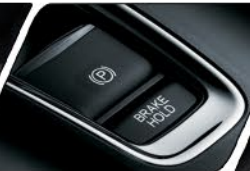
ELECTRIC PARKING BRAKE & AUTO BRAKE HOLD
